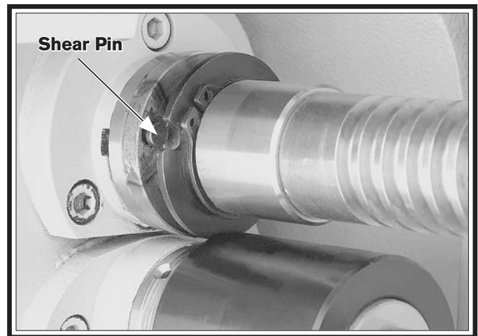
Figure 132. New shear pin installed in bore.
